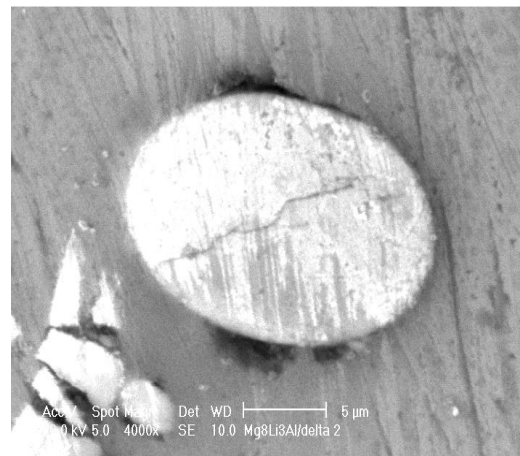
Fig. 7. Typical SEM pictures of microstructures after compression of the Mg8Li3Al/δ AMC composite
