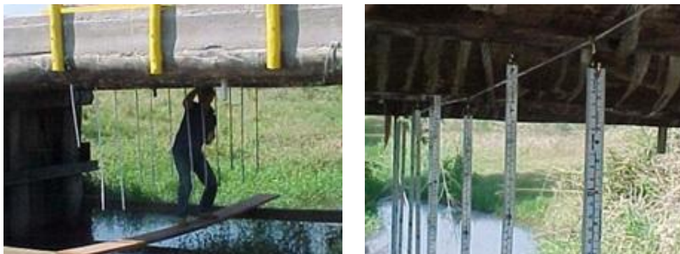
Fig. 11. Positioning of rules for reading vertical displacements at center line of the bridge
