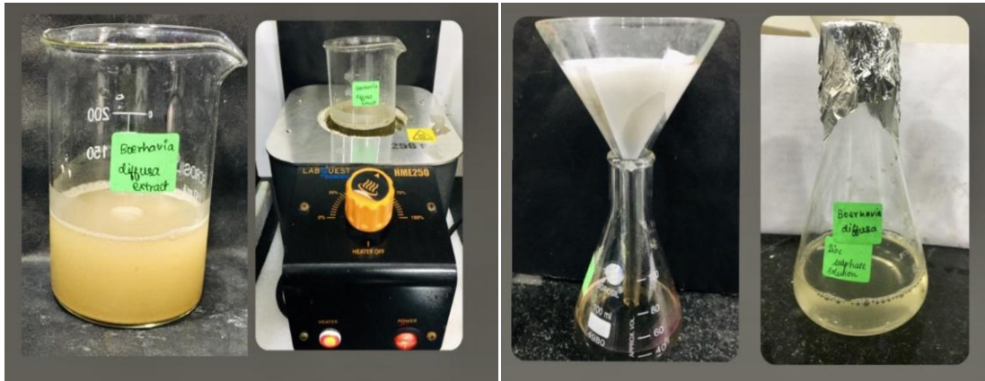
Fig. 1. Preparation of zinc oxide nanoparticle using boerhavia diffusa extract
