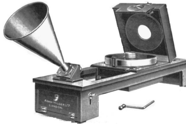
Figure 1. The general appearance of an optical sonometer. Reproduced from [1]. © IOP Publishing Ltd All rights reserved.
