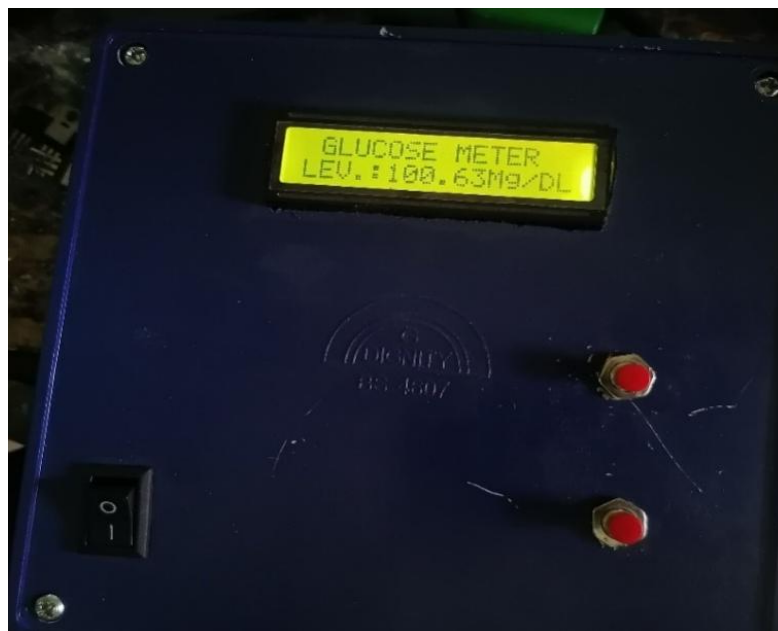
Plate 2. Fabricated glucometer displaying blood sugar result
