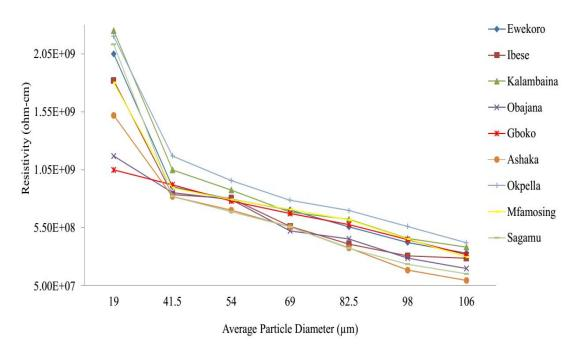
Fig. 4. Resistivity of distinct sizes of particles at ambient temperature (26.5°C)
