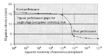
Fig. 1. Effects of particle resistivity on ESP performance [9]
