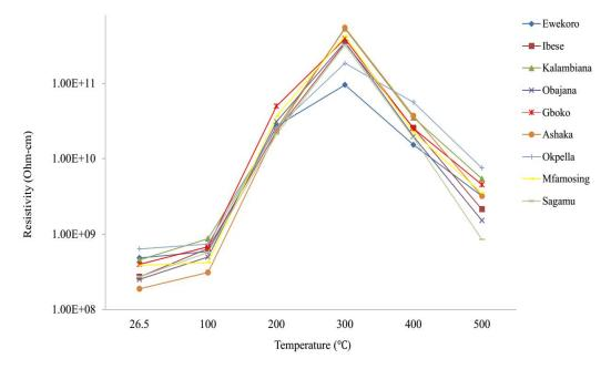
Fig. 3. Resistivity of the samples at varying tegrees of temperature
