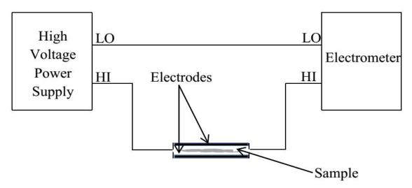
Fig. 2. Circuit configuration for resistivity measurement
