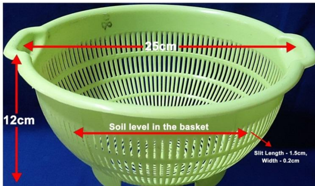
Fig. 1. Dimensions of basket for root angle measurements by basket method
