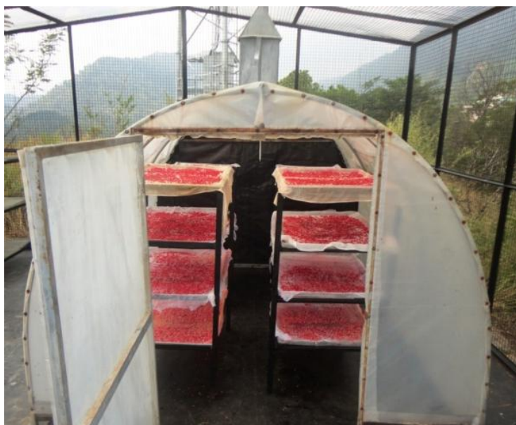
Fig. 1. Drying of wild pomegranate arils for anardana preparation under solar tunnel drier
