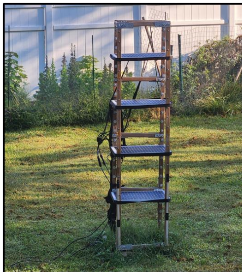
Fig. 2a. Presents the vertical placement of four solar panels with 15 inches of separation
