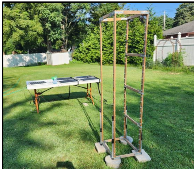
Fig. 2b. Presents the connections of the four solar panels side-by-side with the stacking tower on the side
